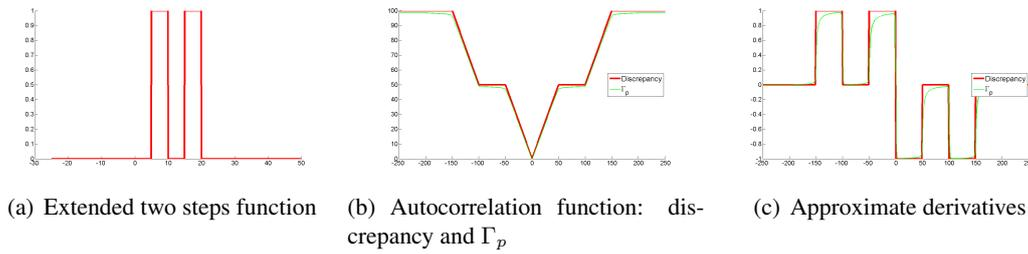
Figure 4: This figure shows how a gradient descent based optimization algorithm might fail when trying to locally optimize the discrepancy correlation function. Indeed the correlation function (second figure) shows some plateau where the derivative (illustrated on the third figure) is 0. On the other hand, using an appropriate  $p$ -norm approximation allows to overcome this effect while keeping a really close objective function.
